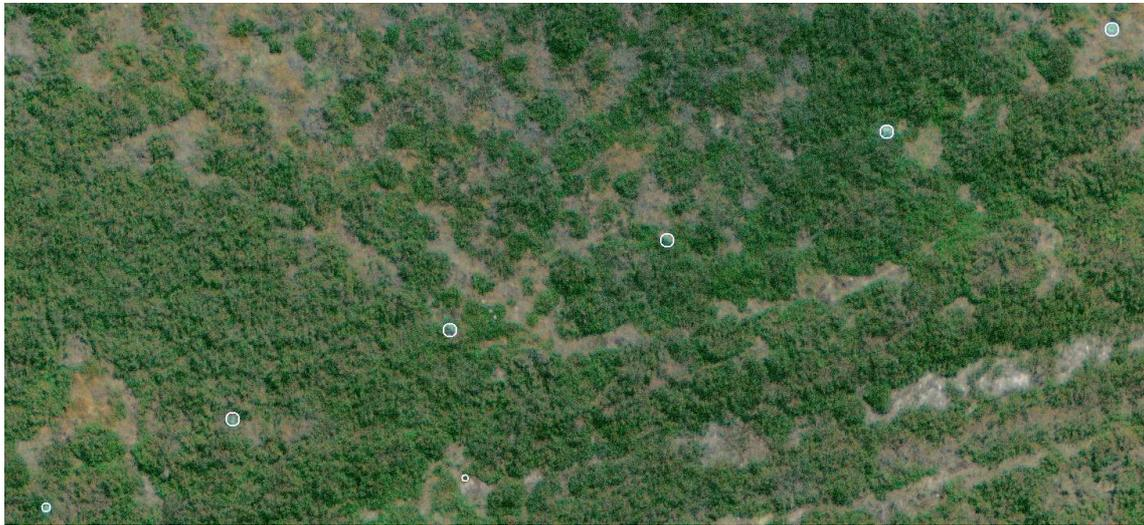
Figure 4.10: Mine-like objects detected on visible image, with what seems to be a false alarm
