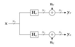
Fig. 1. Gaussian MIMO wire-tap channel
