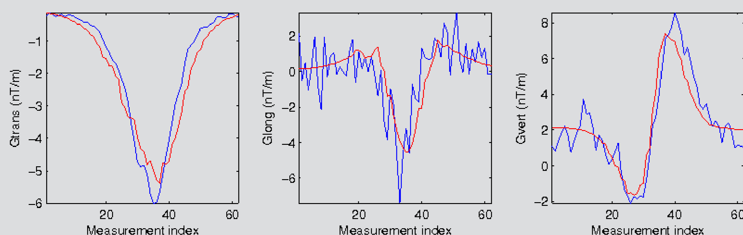
Figure 3: Transversal, longitudinal, and vertical gradients measured (in blue) and for the dipolar model (in red).
