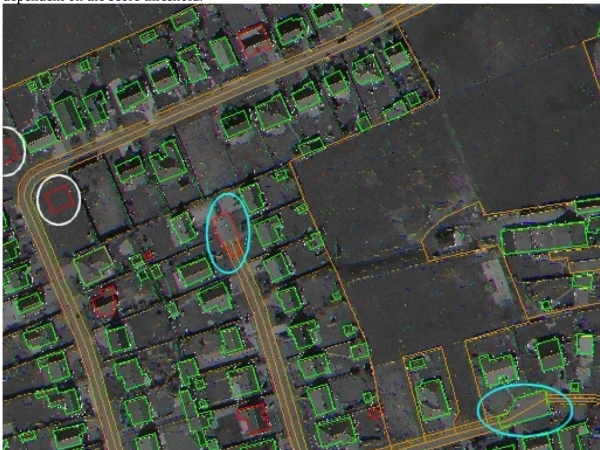
Figure 4. Building verification results: polygons of verified buildings in green and unverified ones in red; blind alleys circled by light blue ellipses and phantom building polygons by white circles.
