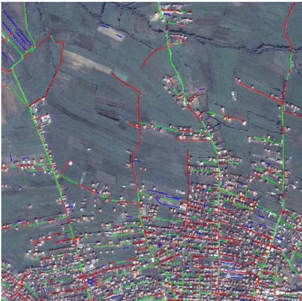
Fig. 3: Extracted roads: Green=correct, Red=missing, Blue=false positive
