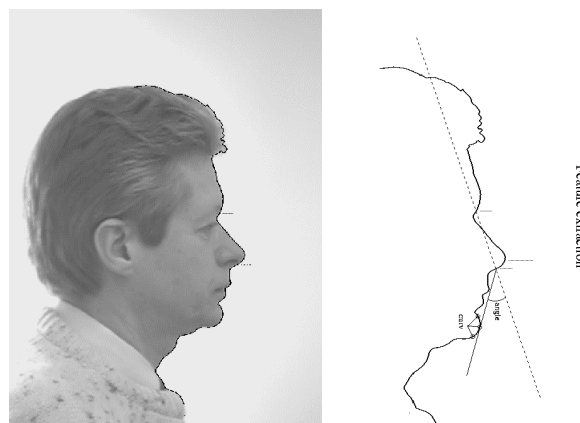
Figure2: a) Profile image b) contour extraction, nose and eye localization, feature extraction
