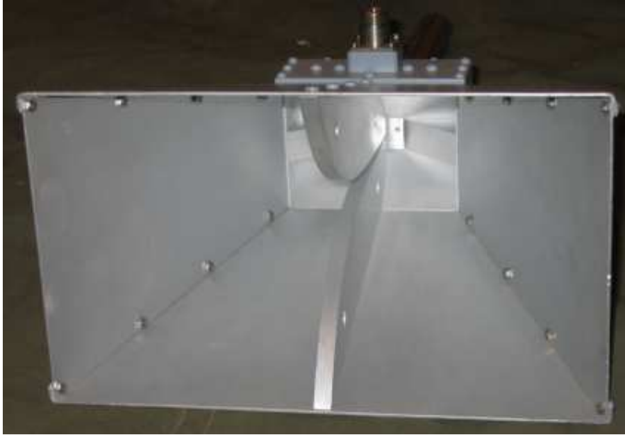
Figure 2.1: Schwarzbeck BBHA TEM ridged-horn ultra-wide band (1–18 GHz) antenna used in the measurements. Aperture size is 24 \text{ cm} \times 14 \text{ cm} .
