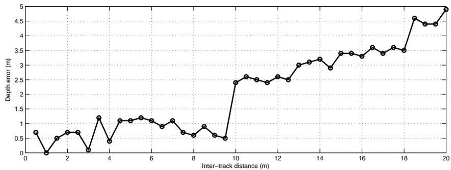
**Fig. 3:** Errors in the estimation of the depth (in metre) as a function of the distance between two tracks (in metre)
