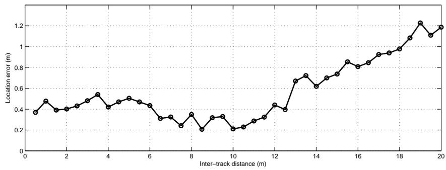
**Fig. 2:** Location errors (in metre) as a function of the distance between two tracks (in metre)
