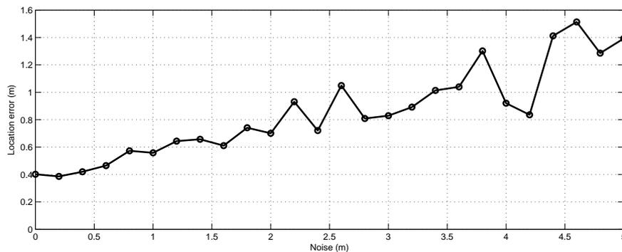
**Fig. 5:** Location errors (in metre) as a function of the noise (in metre)
