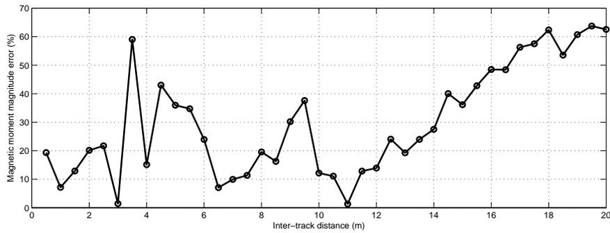
**Fig. 4:** Errors in the estimation of the magnitude of the magnetic moment (in %) as a function of distance between two tracks (in metre)
