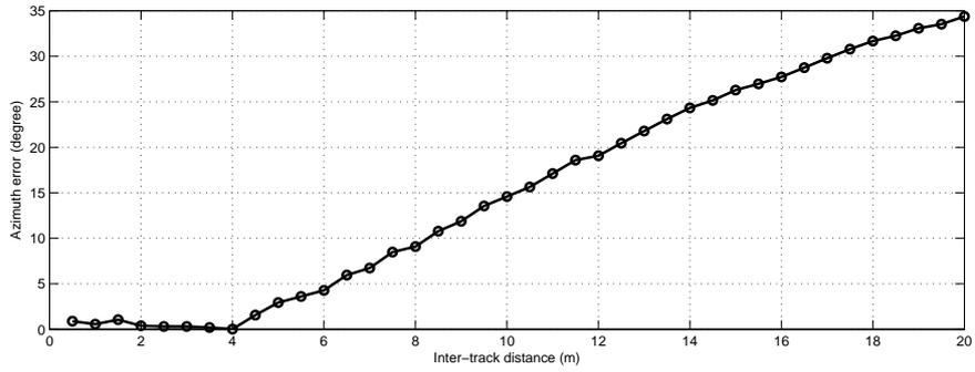
**Fig. 1:** Azimuth errors (in degree) as a function of the distance between two tracks (in metre)
