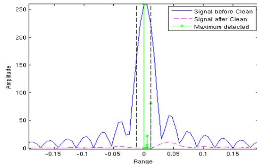
Figure 2: Clean algorithm after 5 iterations and a coefficient of 0.75
