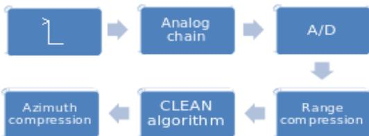
Figure 1: Block diagram of the processing.
