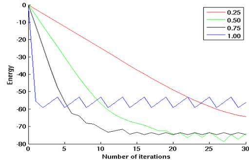
Figure 3: Evolution of sidelobes energy as a function of the iterations for varying coefficients.
