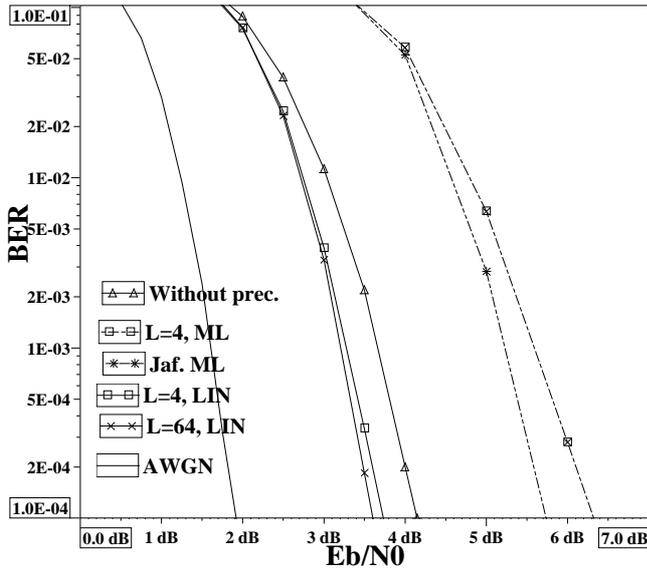
Fig. 3. Performance, with duo-binary turbo channel coding, of OSTBC with Hadamard linear precoding for  $\eta=2$ bps/Hz and 4-transmit antennas
