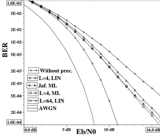
Fig. 2. Performance, without channel coding, of OSTBC with Hadamard linear precoding for  $\eta=2$ bps/Hz and 4-transmit antennas
