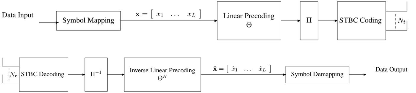
Fig. 1. Linear precoding with OSTBC transmitter and receiver
