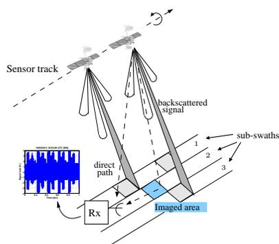
Figure 1: Geometry of the bistatic ScanSAR operating SAR.
