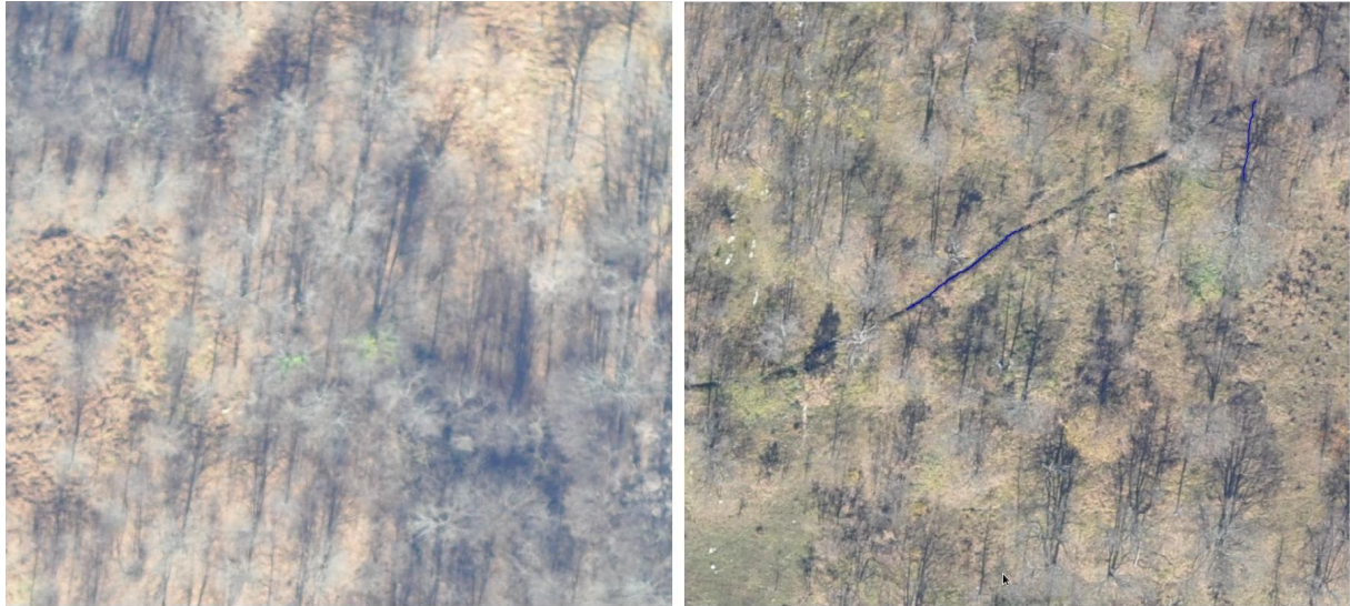
Figure 2. Parts of two color photographs of stripe 1. Left: non suspicious photograph. Right: Most suspicious photograph with linear objects superimposed in blue (min length= 180, min width= 5) .
