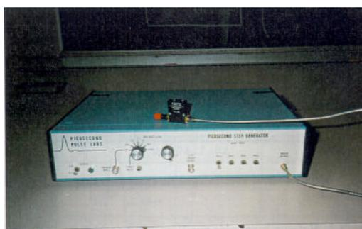
**Fig. 6-2:** The Picosecond Pulse Labs step-generator, type PSPL 4050B
