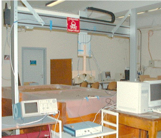
**Fig. 6-7:** Set-up of the UWB GPR system on the indoor xy-table
