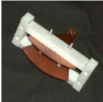
**Fig. 3-18:** Picture of the air-filled TEM horn
