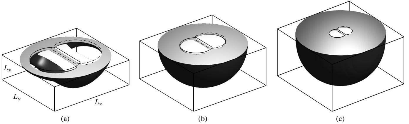
Fig. 4. Smallest VoI and corresponding bounding box for the double-D head with dimensionless height  $h = 0.05$ . (a)  $\alpha = 0.5$ , (b)  $\alpha = 0.90$  and (c)  $\alpha = 0.99$ .  $L_x$ ,  $L_y$  and  $L_z$  are the dimensions of the bounding box along the corresponding axes.
