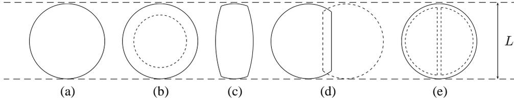
Fig. 2. Head configurations considered. TX — and RX -- coils for (a) circular, (b) concentric, (c) elliptic, (d) double-D and (e) quad heads. For circular and elliptic heads, a single coil is used for RX and TX.  $L$  is the characteristic head length.
