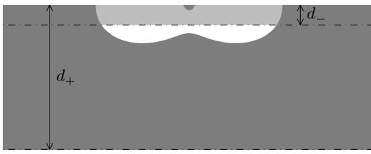
Fig. 3. *Layer of influence* for the double-D head and for a response ratio  $\alpha = 0.95$ . Vertical cut trough the center of the head is illustrated and shows the projection of TX (—) and RX (—) coils, the border of generating volume (— · —), the positive (dark gray) and negative (light gray) layer of influence with corresponding positive and negative depths of influence  $d_+$  and  $d_-$ . The holes in the *layer of influence* appear in white.
