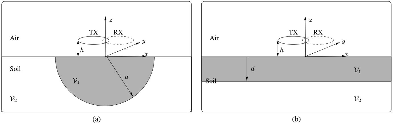
Fig. 1. Two shapes that may be used to define VoI (a) sphere of radius  $a$  and (b) layer of depth  $d$  leading respectively to the half-sphere of influence and to the *layer of influence*. TX (—) and RX (---) coils are shown.  $h$  is the head height above the soil.
