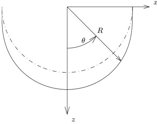
Fig. 6. Shape of the far-field equi-sensitivity (—), and half-circle (---) for comparison.
