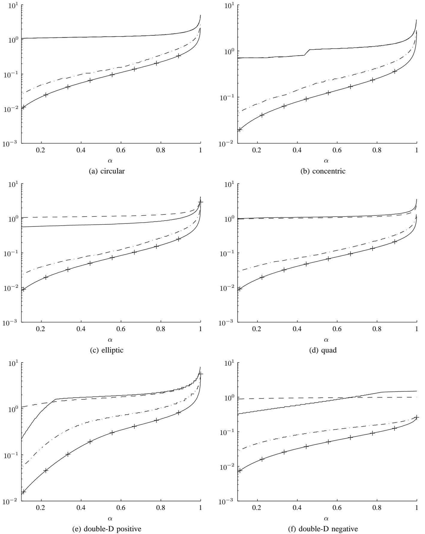
Fig. 7. Size of positive (a-e) and negative (f) VoIs versus fraction  $\alpha$  for circular (a), concentric (b), elliptic (c), quad (d) and double-D (e,f) heads. To characterize the *smallest* VoI, the size of the dimensionless bounding box  $L_x$  (—),  $L_y$  (---) and  $L_z$  (- · -) are shown. To characterize *the layer of influence*, the dimensionless *depth of influence*  $d$  (+) is shown. In all cases, the dimensionless head height is  $h = 0.05$ .
