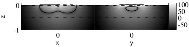
Fig. 3. Vertical XZ (left) and YZ (right) cuts of normalized absolute sensitivity ( $|S|$ ) in dB for double-D head at  $h = 0.05$ . TX (—) and RX (---) coils, depths of horizontal cuts (— · —) as well as zero equi-sensitivity contour (—) are shown.
