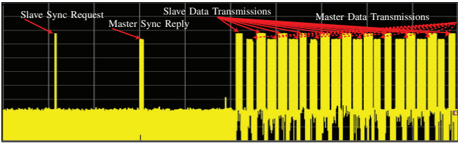
Fig. 5: An example of message-exchange sequence in master/slave setup. Upon receiving sync reply message, slave node is synchronized with the master node. After synchronization, the master and slave nodes exchange data messages according to their slot assignment.
