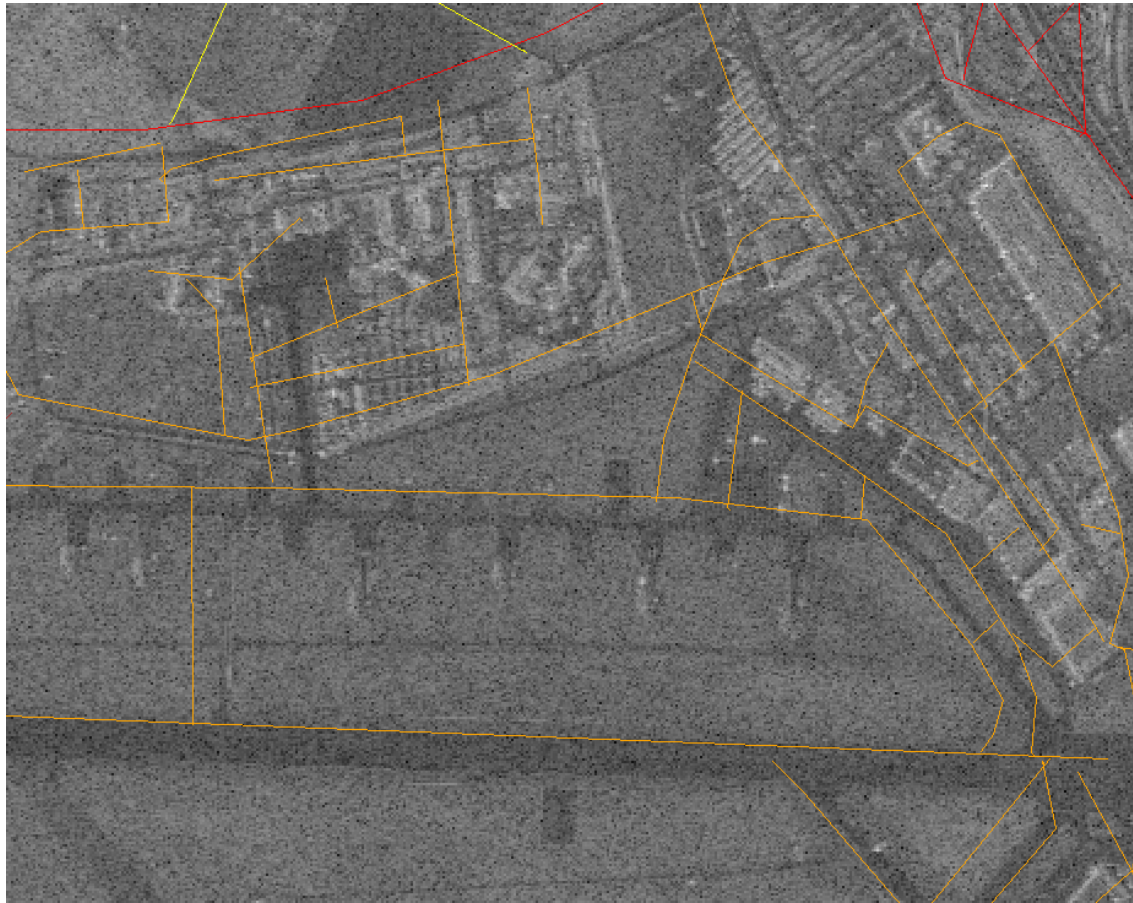
Figure 8.14: Communication lines extracted from the map and projected onto the SAR image
