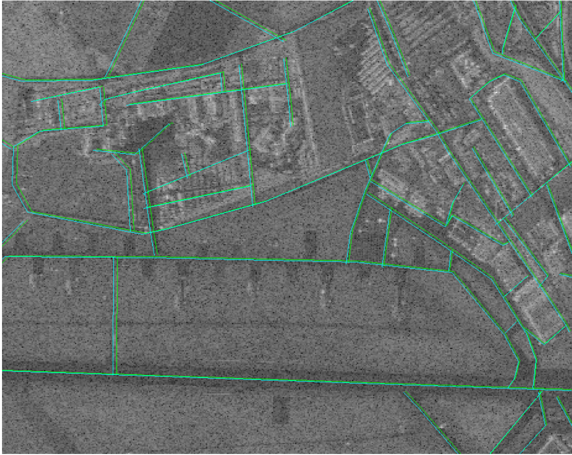
Figure 8.17: Results of the refinement using the simplex method (green) and the LSQ method (cyan)
