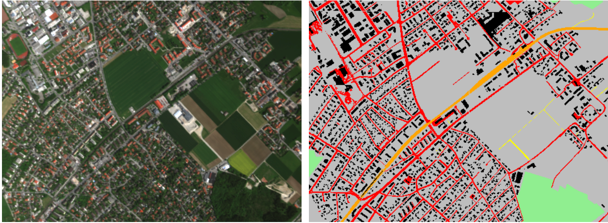
Figure 1: Part of the original hyperspectral data in RGB color composition (left) and ground truth map (right) Legend: red: roads, black: buildings, yellow: paths, orange: railways, green: forests, grey: background
