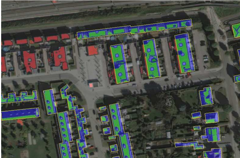
Fig. 2. Classified regions. Green if region in database polygon, Blue for polygon part not verified, Red for candidate regions not in the database
