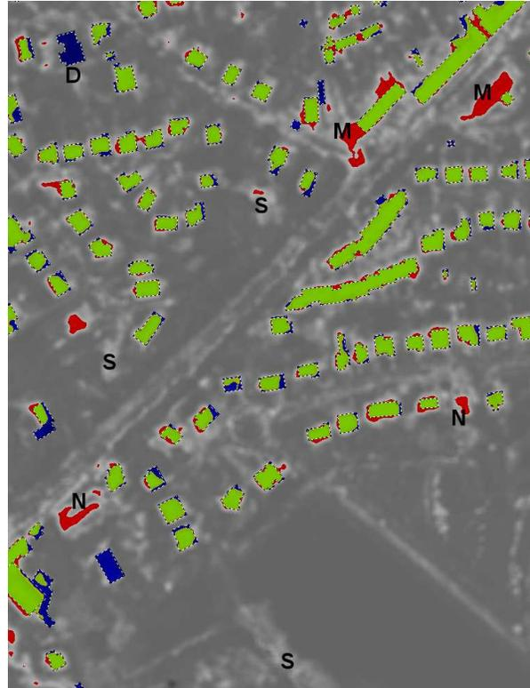
Figure 5: Part of the Building Confidence Map with automatic false coloring: GREEN: confident in DB, RED=confident out of BD, BLUE=not confident in DB. A few examples of New (N), Modified (M) and Disappeared (D) buildings, and Shadow (S) areas.
