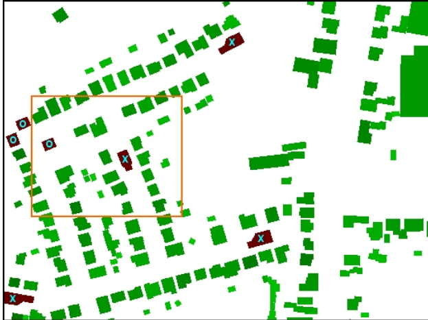
Figure 5. Building verification map. Dark polygons have low scores and should be rejected. The rectangle outlines the area of Figure 3. Blind alleys are marked 'x' and phantoms 'o'.
