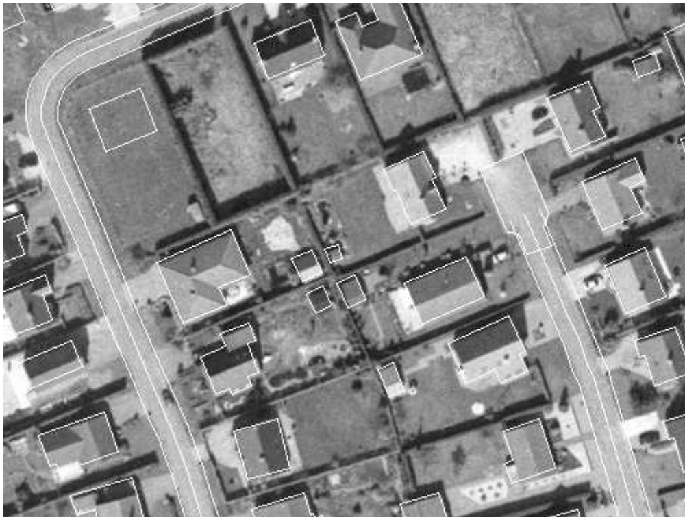
Figure 4: Small part of a test image with superimposed vectors containing one phantom building and one blind alley. Notice the numerous small outbuildings.
