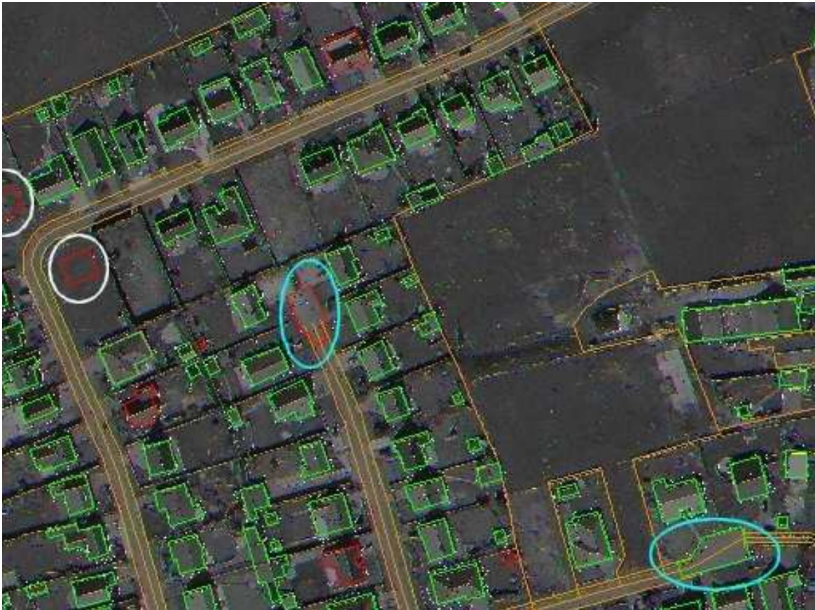
Figure 5: Building verification from edge segments: polygons of verified buildings in green and unverified in red; blind alleys circled by light blue ellipses and phantom building polygons by white circles.
