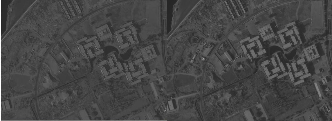
Figure 1. Part of the left and right images of the Ikonos stereo pair.
