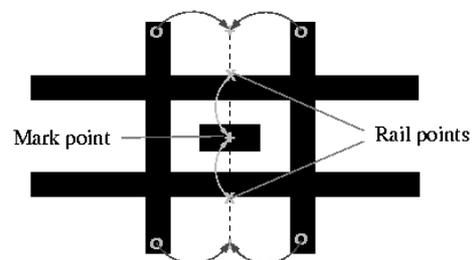
Figure 5 : Localizing rail points
