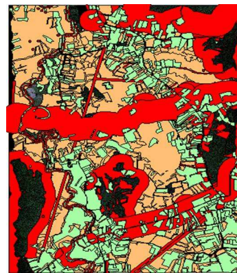
Figure 7: Discrete 'danger map' of Glinska Poljana (preliminary) Red: Danger (Buffers) Orange: Danger (Areas no longer in use) Green: No danger (residential areas, cultivated areas...) Other: No status (forests)
